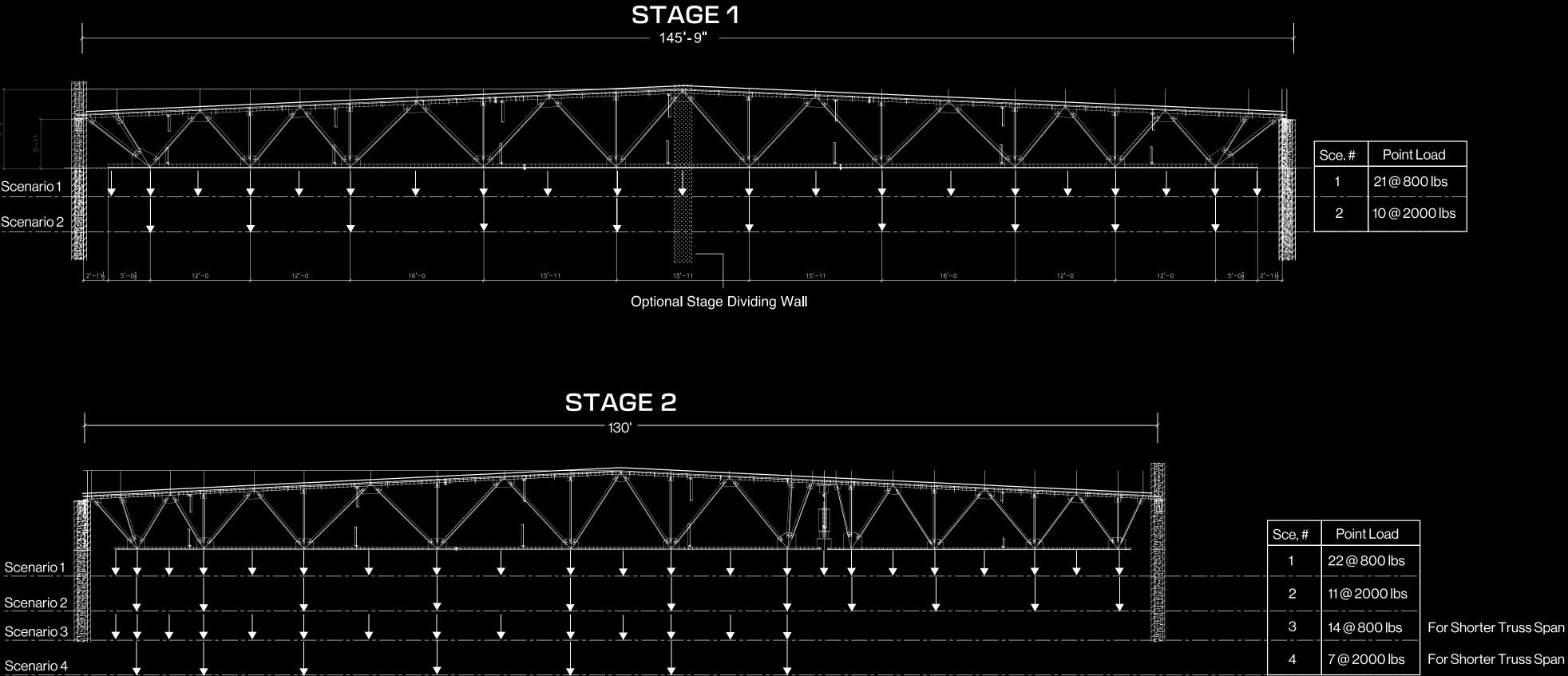
1. Max permissible truss load based on 20 psf.
